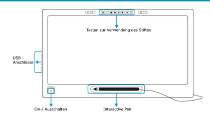
The function of the pen can be controlled via the buttons on the upper edge of the monitor:
